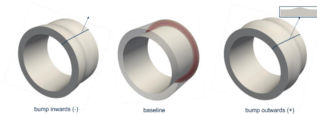
Figure 7. Illustration of different rib configuration on the concentric pipes.
