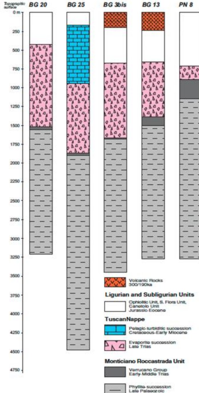
Figure 45: Simplified stratigraphic logs of the indicated geothermal boreholes drilled for geothermal purposes. Some of these are feeding the geothermal power plants of ENEL GreenPower (BG20, BG25, BG3bis, and BG13) whereas the Poggio Nibbio borehole (PN8) is not currently used (from Brogi, 2008).
